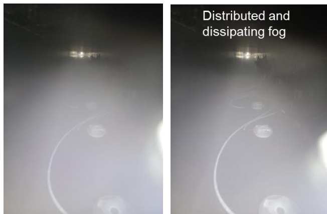
Figures 9d, 9e. The fog in the chamber shows no stratification after some time with circulation
