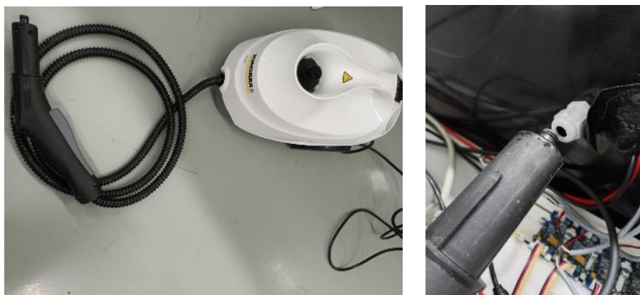
Figures 3a, 3b. Steam cleaner as a fog generation source and inlet opening into the chamber
