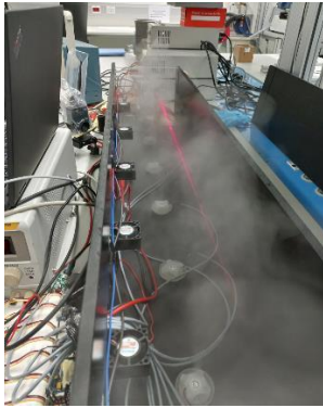
Figure 10a. Picture of the opened chamber with running fog sprayer system and laser beam
