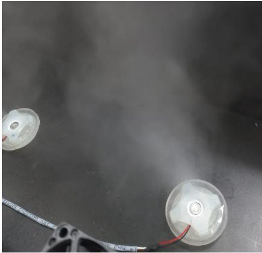
Figure 4. Piezo transducer sprayer unit as a fog generation source
