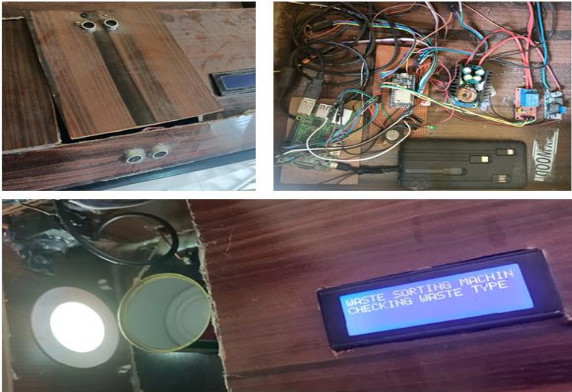
Figure 19. IoT bin – Top view, Circuitry and Display Units – for Solid Waste Classification using CitewasteRN50 model
