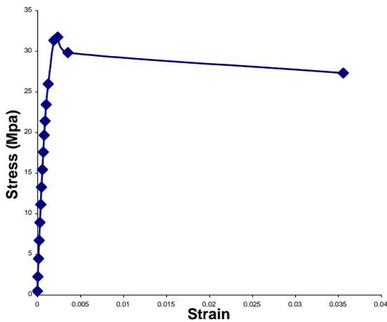
Figure 5a: Stress-Strain response at 216 mm from top
