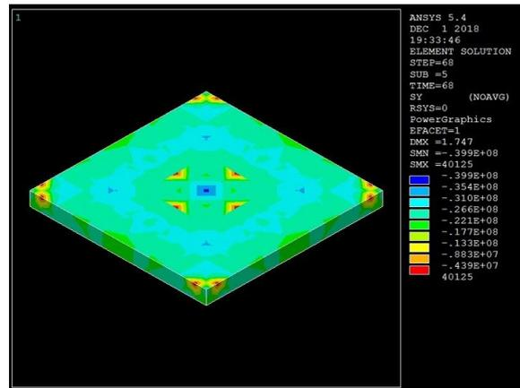
Figure 6b. Stress distribution pattern at 432 mm from top
