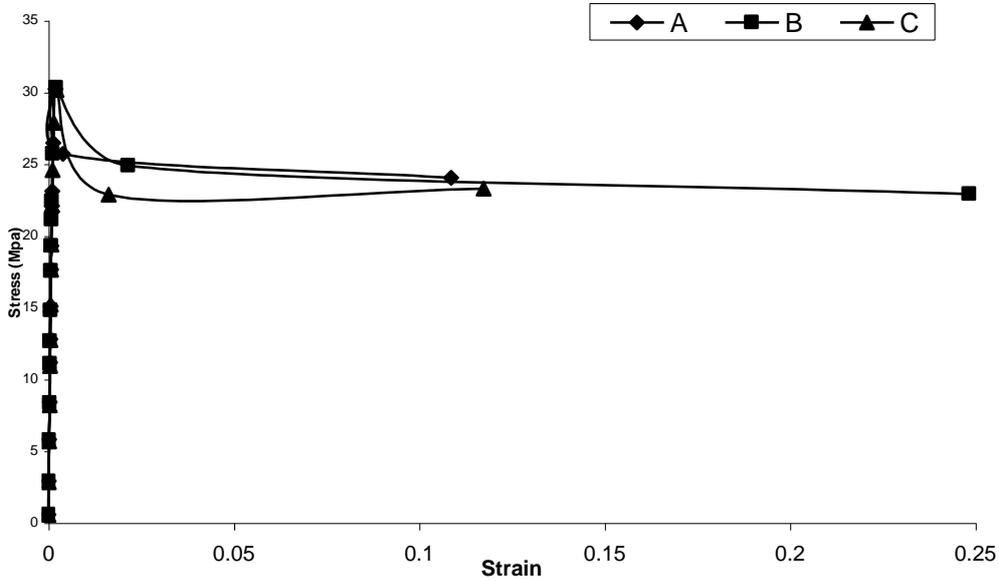
Figure 8. Stress – Strain responses for different tie arrangements at middle of central region
