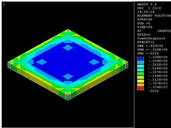
Figure 6a. Stress distribution pattern at 216 mm from top
