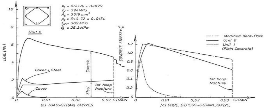
Figure 4. Load-Strain & Stress-Strain curves of the experiments by Scott (Source: Scott, 1980)
