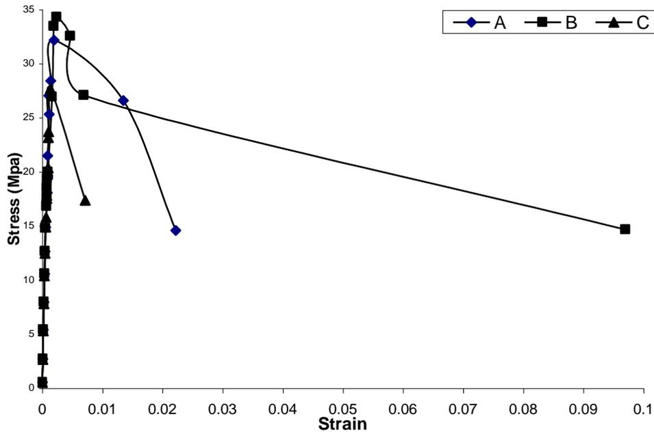
Figure 9. Stress – Strain responses for different tie arrangements at the edge of central region
