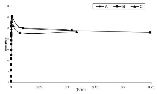
Figure 8. Stress – Strain responses for different tie arrangements at middle of central region
