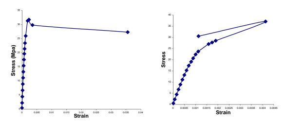
Figure 5a: Stress-Strain response at 216 mm from top
