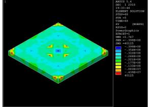
Figure 6b. Stress distribution pattern at 432 mm from top
