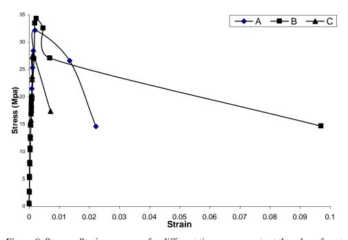
Figure 9. Stress – Strain responses for different tie arrangements at the edge of central region
