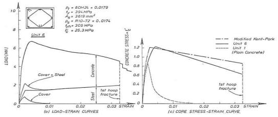
Figure 4. Load-Strain & Stress-Strain curves of the experiments by Scott (Source: Scott, 1980)
