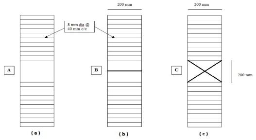
Figure 7. Columns with different tie - arrangements selected for comparative study
